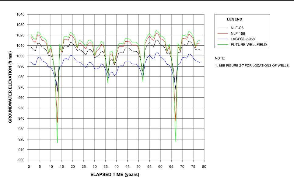
FIGURE 2-15 SIMULATED AVERAGE ANNUAL GROUNDWATER ELEVATIONS IN THE SAUGUS FORMATION WEST OF INTERSTATE 5
