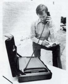
BETTER THAN AGENT 007. You can be the owner of a Mark 900 Attache Phone. Concealed within this top grain leather briefcase is a self-contained antennae, puch button control panel, conference speaker and combination lock for security. The phone itself is solid state, has eleven channels and automatic dial capability. It is completely portable, weighing approximately 14 pounds, with re-chargeable NiCad batteries, it can be used anywhere for the busy business man who needs instant communication.
